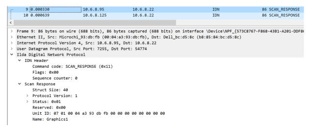
The IDN unit ID is like a globally unique serial number and can be used to unambiguously distinguish between different IDN units (devices) and, moreover, recognize devices in a local network even if the IP addresses have changed. The host name is a human user friendly name to identify the IDN unit. In the Wireshark trace, unit names like Left3, Left2, ..., Center, Right1, Right2, ..., Graphics1 are used.
