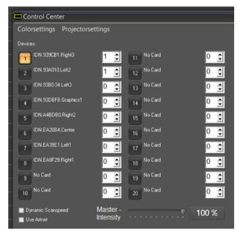
A software system can make use of the information returned from IDN scan response and service map response and can display this information to the user of the software, e.g. here in the menu to select color and projector settings. In this case, each IDN device is identified by e.g. "IDN.93DBFB.Graphics1" which contains part of the IDN unit ID and the IDN service name.
