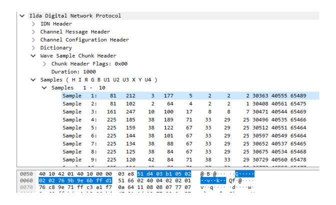
As recommended by [IDN-Stream, section 2.2] a configuration header is repeatedly contained in the IDN channel message and thus visible in the Wireshark trace again after about 250 ms, i.e. every 250<sup>th</sup> message in the trace carries the configuration header with the dictionary.
