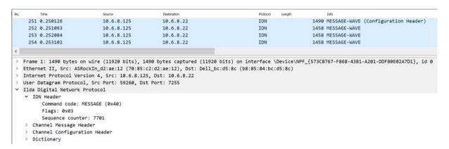
The payload of each IDN datagram begins with the IDN-Hello packet header of 4 byte length. All IDN stream datagrams presented in this section have the command code 0x40 (Realtime stream: channel message). Cf. section 2 of [IDN-Hello].
