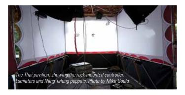
of blue at 445nm. To achieve a wide spread at such a short throw (~9'), the Lumiators are fitted with diverging lenses, bought surplus and originally intended for TOW anti-tank missile nose cones.
