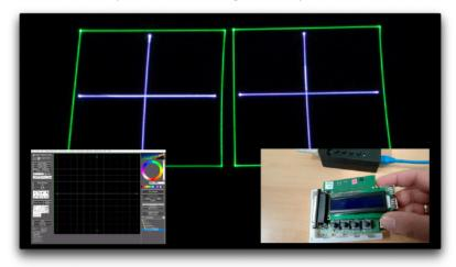
This IDN award entry is about IDN consumers for Laser Projector and DMX512 Service. For each service, a low-cost device composed of off-the-shelf hardware components receives a network data stream according to the IDN stream specification and is able to generate the appropriate electrical control signals for ILDA ISP-DB25 (Laser Projector Service) or DMX512.
