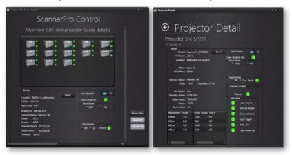
Live Feedback is laser industry oriented data acquisition hardware and software created to monitor and control up to 30 laser projectors. This control can be used with the same Ethernet cable used to send laser graphics to the projectors.
