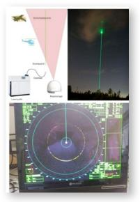
It has a range up to 90 nautical miles and can also be used at bad weather. A filter does not activate the alarm during cloudy or rainy conditions. The detecting cone angle is 20° in the standard version. The radar emitter is unlike rotating radars, instead being a horn-emitter that has especially been designed for this application. Unlike a rotating radar there is no interruption of signal. It is constantly detecting the airspace.
